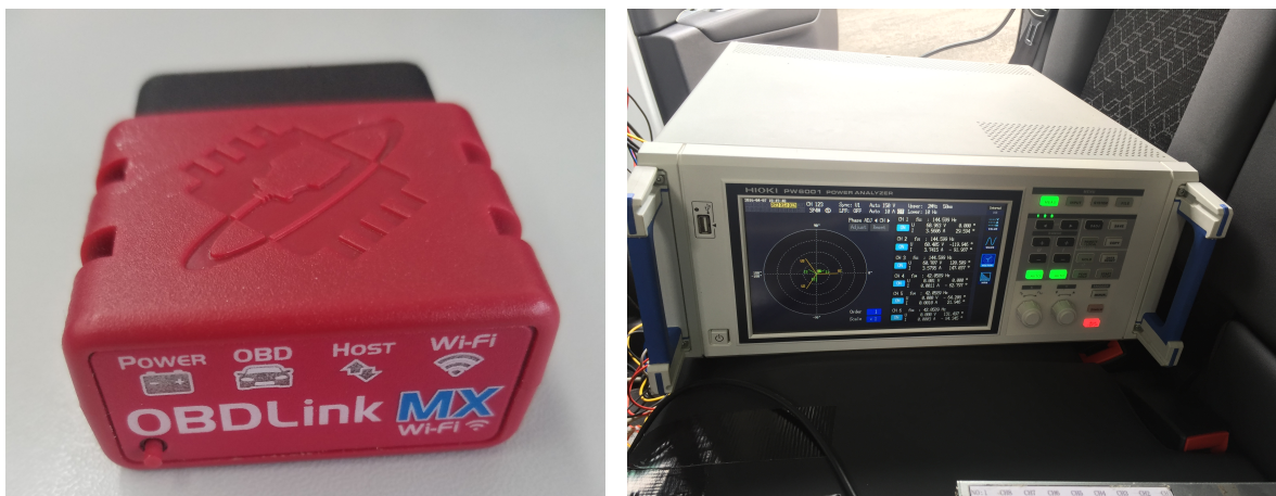
Figure 4. Energy consumption data logging tools: OBD tool (left) and power analyzer (right).
